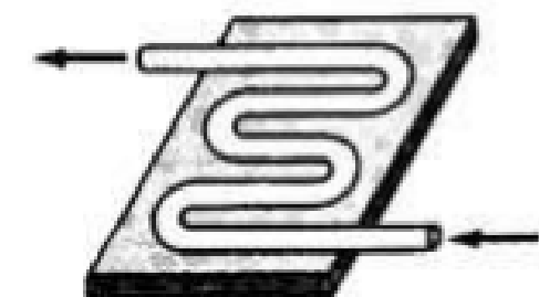
"Serpentine" (metal tubing soldered to metal sheet)
